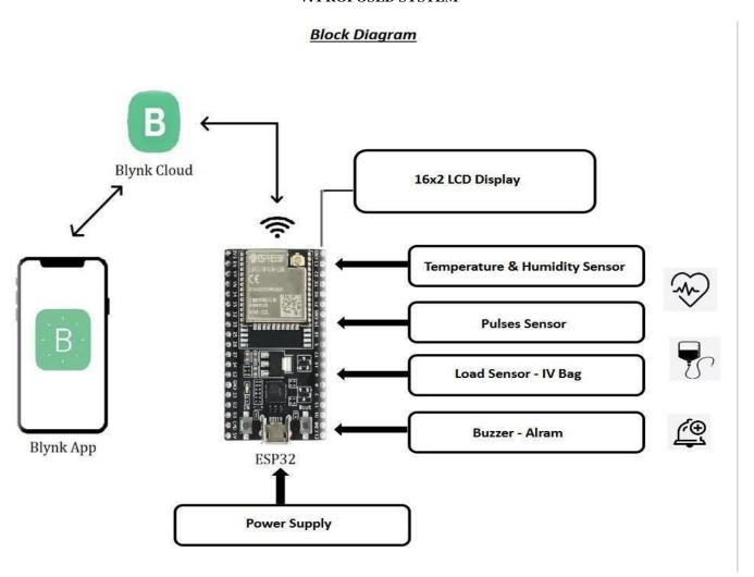
Our system, which uses the ESP32 as its central processing platform, incorporates a number of sensors to keep an eye on things like IV bag weight, patient vital signs, and temperature. Healthcare providers can react quickly to any variation from normal conditions by using the MQTT protocol to generate and transmit real-time notifications. Devices installed in different systems can be connected over the internet thanks to the Internet of Things.
